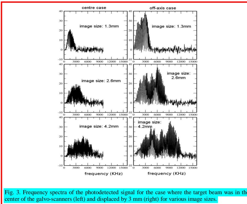
Fig. 3. Frequency spectra of the photodetected signal for the case where the target beam was in the center of the galvo-scanners (left) and displaced by 3 mm (right) for various image sizes.
