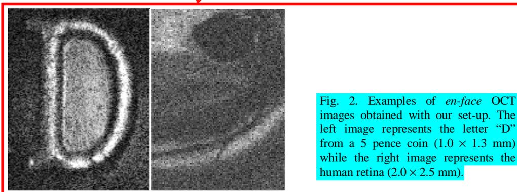
Fig. 2. Examples of *en-face* OCT images obtained with our set-up. The left image represents the letter "D" from a 5 pence coin ( $1.0 \times 1.3\ \text{mm}$ ) while the right image represents the human retina ( $2.0 \times 2.5\ \text{mm}$ ).
