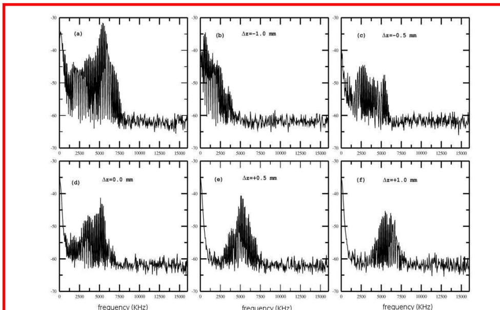
Fig. 5. Frequency spectra of the photodetected signal. The case a corresponds to a situation where the beam was in the centre of the RS ( $\Delta z=0$ ) and its diameter 3 mm while the other cases correspond to a beam diameter of 1.75 mm and various position of the beam on the RS.
