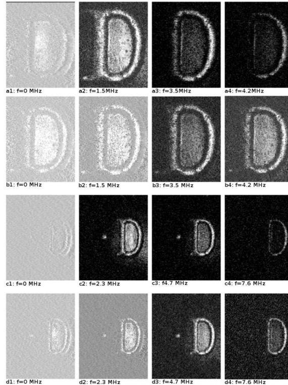
Fig. 4. *En-face* images of a coin obtained while the SA was tuned at various frequencies. The cases a and b correspond to a dimension of 1.0x1.3 mm while c and d to 2.0 x 2.6mm. For the cases a and c the SA bandwidth was tuned at 1 MHz, while for b and d at 3 MHz.
