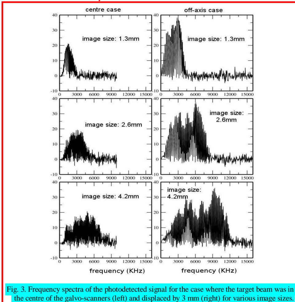
Fig. 3. Frequency spectra of the photodetected signal for the case where the target beam was in the centre of the galvo-scanners (left) and displaced by 3 mm (right) for various image sizes.
