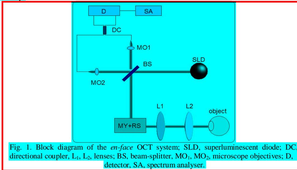
Fig. 1. Block diagram of the *en-face* OCT system; SLD, superluminescent diode; DC, directional coupler, L<sub>1</sub>, L<sub>2</sub>, lenses; BS, beam-splitter, MO<sub>1</sub>, MO<sub>2</sub>, microscope objectives; D, detector, SA, spectrum analyser.
